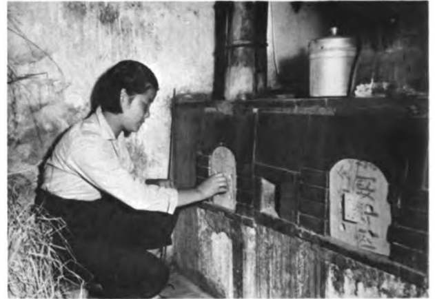
Adding a door to the firebox of an improved stove saves fuel. This Taiwanese girl has covered the inside of her wooden door with tin.
