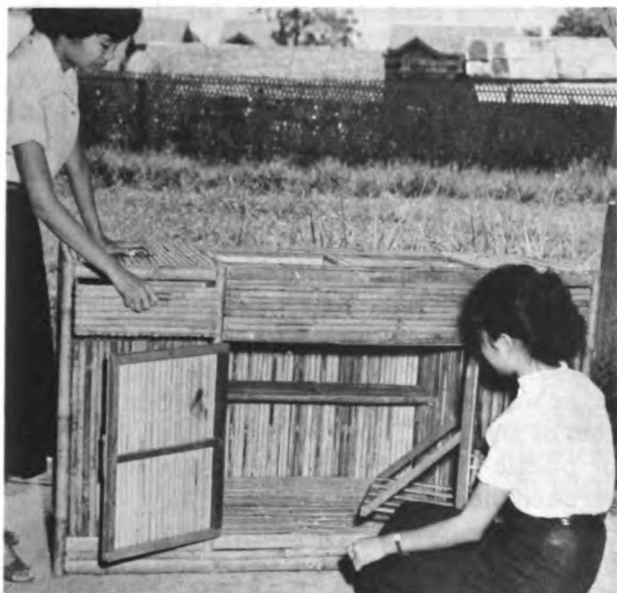
Attractive cupboards can be made of bamboo where it is plentiful. These Thailand workers show drawer, shelf, and sink space in a kitchen unit.
